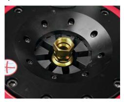
Place the fitting over the fitting adapter.
