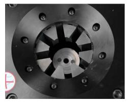
Note that there are 2 powerful magnets in the base to assure that the fitting adapter does not get removed with the fitting at the completion of the crimping cycle.
