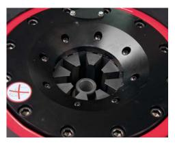
Insert the correct fitting adapter into the base of the machine.
