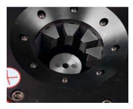
Insert the die fingers into the master die. Note that the dies are sequentially stamped. Insert the dies in the proper sequence.
