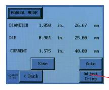
• Due to variations in hose and fitting tolerances a minor crimp adjustment may be required if the measured diameter of the final crimp is not within the hose and fitting manufacturer's specifications. ACT™ technology makes minor corrections a simple process which requires no addition or subtraction.
