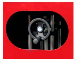
Adjust the fitting up or down until the nut crimping dies are in the correct position relative to the fitting.
