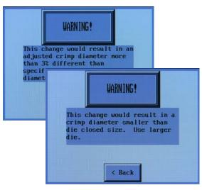
• If an operation is attempted which is outside of the range of the die set selected or which could result in a bad crimp, a series of warning screens will appear to help diagnose the problem.
