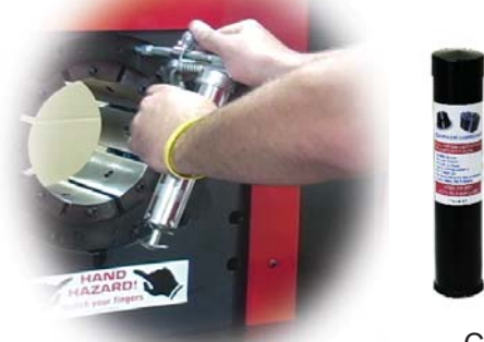
Die Lubrication with CrimpX
