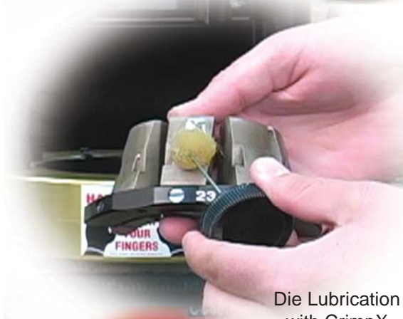
Die Lubrication with Moly Disulfide Grease
