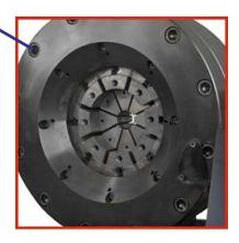
Proper lubrication is essential to prevent damage to the machine and to assure accurate crimping.
