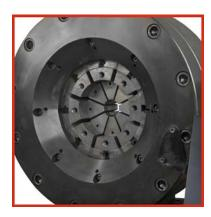
Do not lift the machine by the crimper head. Lift with a fork lift under the tank.
