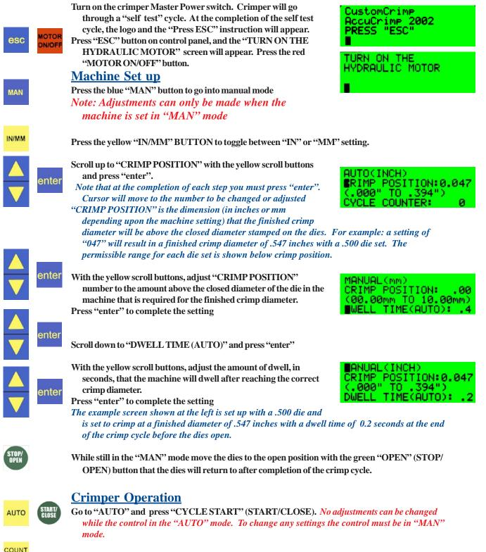
The cycle counter can be reset at any point to maintain a running count of crimp cycles.
