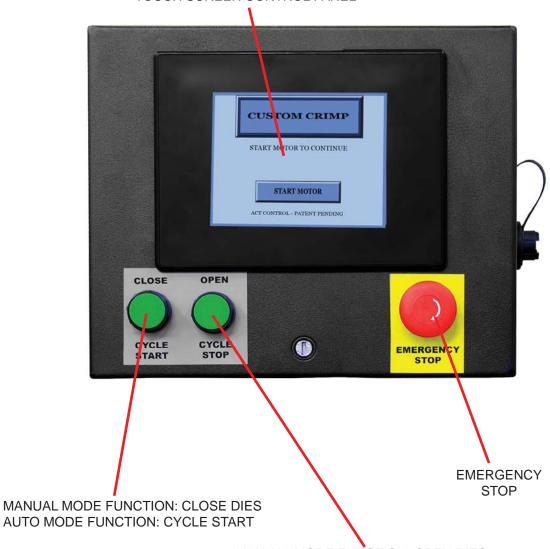
MANUAL MODE FUNCTION: OPEN DIES AUTO MODE FUNCTION: CYCLE STOP
