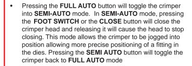
In **FULL AUTO** mode pressing the foot switch will start the crimp cycle and the dies will stop closing when the crimp cycle is complete
