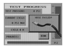
If the test does not complete satisfactorily, the Hose Failed screen will appear.
