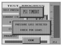
Test cycle was unable to finish due to pressure leaks.
