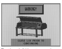
Test bench lid is not properly closed and latched.
