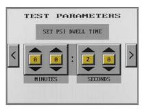
Set the time for the hose to be held at test pressure.
