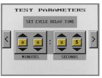
Enter the delay time between test cycles.
