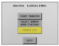
Select Remove USB once transfer completes. Exit and remove Flash Drive from control panel.
