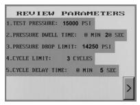
Review test parameters prior to running test.
